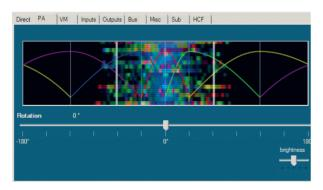
The PA window features a visualization of the Panoramic Analyzer's dynamic filtering with overlapping filter bands. The angle set in the PA parameter section is represented by two light grey vertical lines. A vertical spectrogram of the incoming stereo source is shown between these lines.
