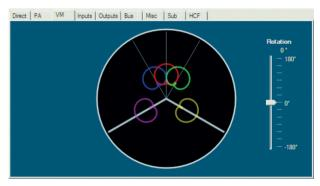
The VM window features a graphic representation of the virtual 5.0 microphone setup used by the VM module. The angle set in the VM parameter section is represented by two light grey lines; the form of the virtual microphones show the polar pattern set with the "Lobes" parameter.
