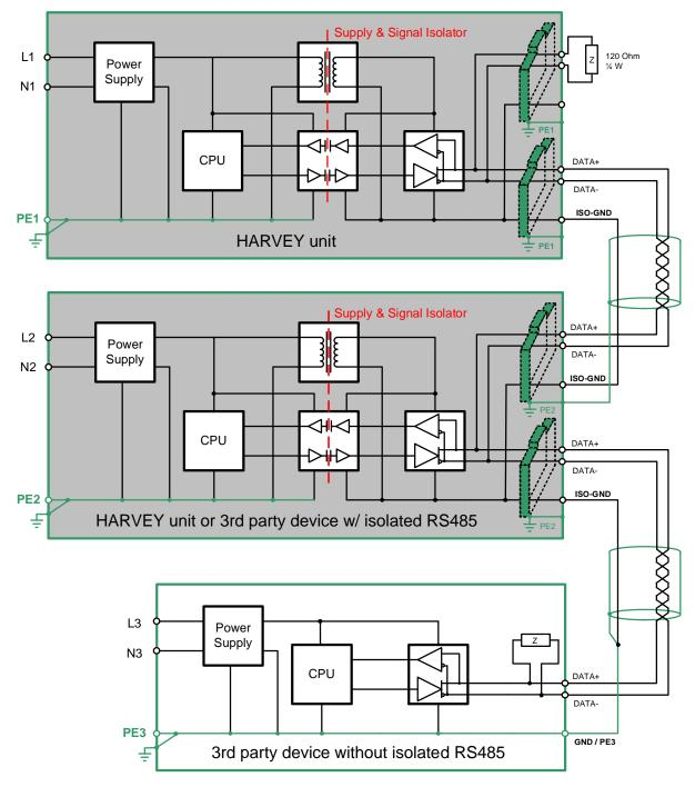
Internally the RS-485 circuit is carried out isolated with regard to signals and power supply. This structure avoids ground loops which may occur in systems with long distances between the protective earth (PE) -grounding points and which may lead to communication faults. Each RS-485 interface of HARVEY offers a ground signal which is isolated from PE-ground. Only the RJ45-shield is connected to the PE-grounded device housing.
